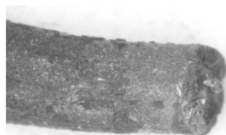
图6 主回路连接线位于螺栓侧断口 Fig. 6 The main circuit connection line located at the bolt side fracture
