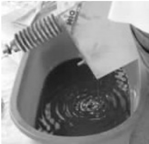
图6 8号电容器放浸渍液 Fig. 6 Drainage of impregnating solution of 8# capacitor
