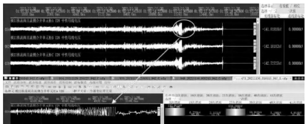
图6 FK站分压器故障波形 Fig. 6 Fault waveform of voltage divider of FK station
