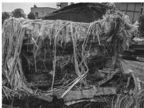
图5 第1至第6包封层烧损情况 Fig. 5 Burn-off condition of the 1st to the 6th encapsulation layers
