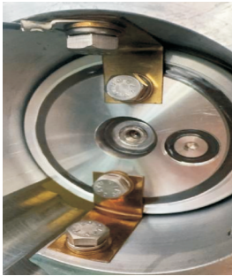
图6 2处连接片均断裂 Fig. 6 Breakage of two connection pieces
