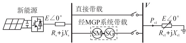
图5 基于P-V曲线法的光伏系统结构图 Fig. 5 Structural diagram of PV system based on the P-V curve method
