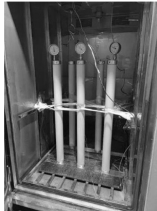
图5 样品在高低温箱内进行试验 Fig. 5 Test of sample at hot and cold temperature chamber
