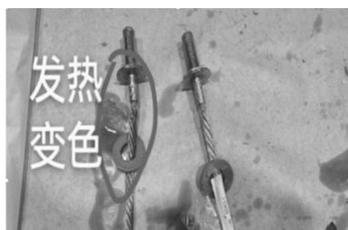
图9 出线套管铜绞线颜色对比 Fig. 9 Color comparison of copper stranded wire of outgoing bushing
